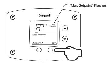
Step 3: Press the "UP" or "DOWN" buttons to change the maximum setpoint value. This will limit the maximum setpoint the user can select. Note: The maximum setpoint is approximately 180°F.
